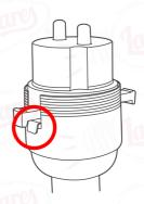
**Step 6:** Ensure you use the cord grip on the bottom of the light fitting by putting it across the cable and using the screws supplied to fix it into position, this will ensure the cable cannot be pulled out by accident.
